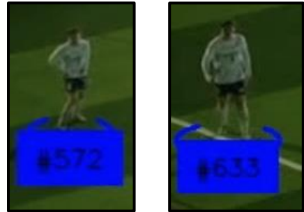
Figure 13. Labeling using ByteTrack only. Left: Player before leaving the frame. Right: Player after rejoining. The label is not the same.
